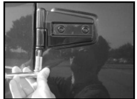
3. Loosely attach Hinge Pin Brackets to the Tube Door using supplied M8 hardware.
