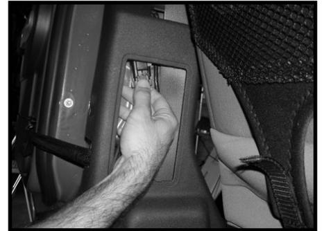
2. Remove the torx nut from the bottom of each factory hinge pin. Set these nuts aside to be re-installed on the Tube Doors. To remove the factory doors, carefully lift the door upward until the hinge pins completely clear the hinges. It will be helpful to have someone else assist with this step.
