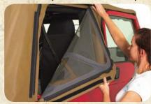
Jeep® applications (and late model Suzuki) feature zip out windows for the true open air experience. Each side and rear window have durable zipper attachments covered by weather seals to keep the weather out
