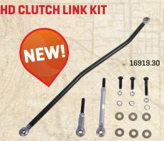
Replaces the factory style L-bracket with retainer clip clutch rod with an upgraded spherical rod design. Allows for full clutch engagement during heavy body and frame flex situations while off road, where the factory design has tendencies to bind not allowing you to get into gear. Also can be used with up to 3" body lifted vehicles replacing the shorter factory clutch rod.
